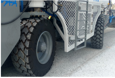
All Wheel Drive Propulsion System Independent Front and Rear Wheel Steering
